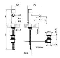
Basin mixer with waste and connecting flexibles. TRAME
