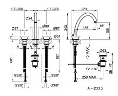
Three-holes medium version basin mixer with waste and connecting flexibles. Can be combined with inserts with different finishes: art. 66600 and art. 66602.
