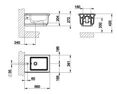
Wall hung bidet in in Ceramic with overflow waste, with central hole for taps and fittings. Overflow cap and side covering caps included in 031 finishing
