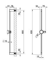
Sliding rail. Can be combined with inserts with different finishes: art. 66600 and art. 66602.
