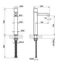
High version basin mixer without waste and connecting flexibles. RIGATO
