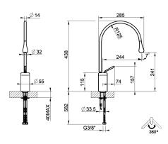
Medium version basin mixer, medium spout, flexible connections, without waste. Swivelling spout.
