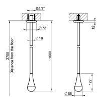
Ceiling-mounted spout to be completed with separate control
