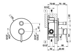
External parts for wall-mounted mixer two-way, automatic bath/ shower diverter
