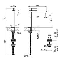
Medium version basin mixer with Stop&Go waste and connecting flexibles. RIGATO.
