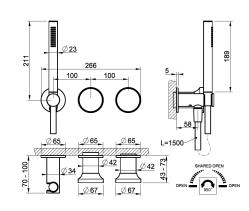
External parts wall-mounted two-ways shower mixer, with diverter, water outlet and hand shower hook. Can be combined with inserts with different finishes: art. 66600 and art. 66602.
