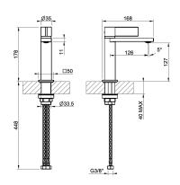
Basin mixer without waste, with connecting flexibles. DIAMANTATO.
