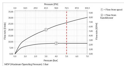
MOP (Maximum Operating Pressure): 5 bar Flow rate is referred to mixed water temperature of 38°C.
