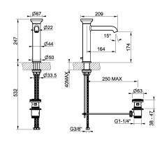
Medium version basin mixer with waste and connecting flexibles. Can be combined with inserts with different finishes: art. 66600 and art. 66602.
