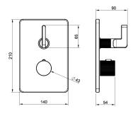
External parts for thermostatic mixer, two-way diverter
