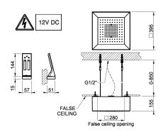
300X300 Built-in shower system, with rainfall function and chromotherapy effect, for ceiling/false-ceiling installation. Electronic parts included with remote watertight control and hook. To be matched with 12V RIR5402 power supply, not included. To be completed with cover (not included).
