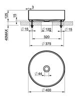
Counter washbasin Ø400mm in stainless steel RIGATO, without overflow waste. Waste not included. It can be combined with waste 54599.
