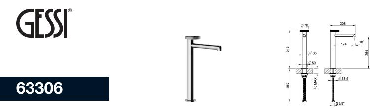
Tall single lever washbasin mixer without pop-up assembly• Spout projection 6-7/8" • Height 12-9/16" • Drain not included - See DRAINS section • Max flow rate 1.2 GPM • ADA compliant
