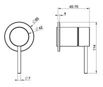
TRIM PARTS ONLY Wall-mounted washbasin mixer control • For spouts 54499 or 54496 • 1/2" connections • Drain not included - See DRAINS section • Requires in-wall rough valve 53112 • ADA compliant • Handle kit
