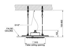
350x350 shower system for false-ceiling installation. With RAINFALL function. To be completed with cover
