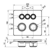
TRIM PARTS ONLY External parts for thermostatic mixer for three functions, with push-button on/off control• Single backplate• 1/2"connections• Anti-scalding• Requires in-wall rough valve 63001• Non-Shared Function
