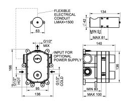
Built-in part for wall-mounted electronic separate control
