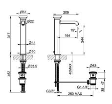
High version basin mixer with waste and connecting flexibles. Can be combined with inserts with different finishes: art. 66600 and art. 66602.
