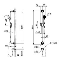
Sliding rail with antilimestone handshower, 1,50 m flexible hose and water outlet
