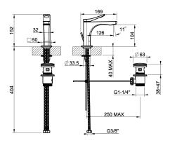
Basin mixer, flexible connections, with waste. Ø25 mm cartridge
