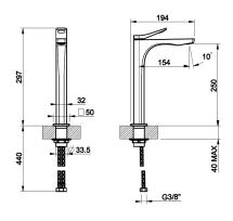
Tall single lever washbasin mixer without pop-up assembly• Spout projection 6-1/16" • Height 11-11/16"• Drain not included - See DRAINS section • Max flow rate 1.2 GPM • ADA compliant
