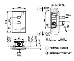
External parts for wall-mounted mixer two-way, automatic bath/ shower diverter
