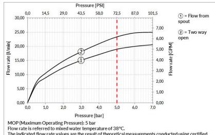
The indicated flow rate values are the result of theoretical measurements conducted using certified laboratory instruments.
