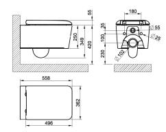
Wall hung WC (6 litres) in Ceramic. Soft-closing hardware included in 031 finishing
