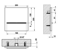
Wall-fixing cascade shower spout to be completed with separate control (not included)
