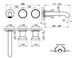
External part for wall-mounted bath mixer, two-ways diverter. Can be combined with inserts with different finishes: art. 66600 and art. 66602.
