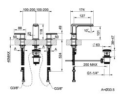
Three-holes basin mixer, with flexible hoses with waste
