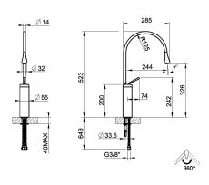
High basin mixer, medium spout, flexible connections, without waste. Swivelling spout.
