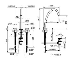
High version three-holes basin mixer with spout, connecting flexibiles, with waste. Can be combined with inserts with different finishes: art. 66600 and art. 66602.
