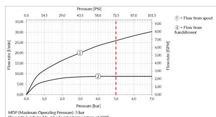
Flow rate is referred to mixed water temperature of 38°C.
