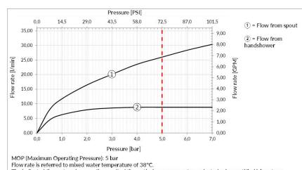
The indicated flow rate values are the result of theoretical measurements conducted using certified laboratory list trumpets.
