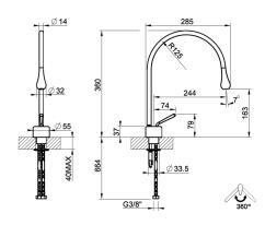
Basin mixer, medium spout, flexible connections, without waste. Swivelling spout.
